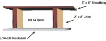
of the joist. ALL R-VALUES ARE SYSTEM R-VALUES. AN ENCLOSED AIR SPACE MUST BE MAINTAINED TO ACHIEVE THESE VALUES. IF THE BOTTOM SURFACE OF THE LOW-E INSULATION MUST BE COVERED BY ANOTHER SURFACE, R-VALUE MAY BE LOWER. Measure entire joist area to determine square footage of ESP Low-E<sup>®</sup> Insulation required(length x width). Roll out material and fasten to bottom of floor joist with 1/2" staples every 6". To achieve a vapor barrier, all seams must be taped securely with Low-E tape.
