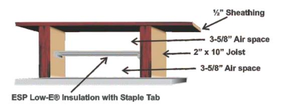
SYSTEM R-VALUES FOR THESE INSTALLATION METHODS WERE CALCULATED USING DATA FROM THE ASHRAE HANDBOOK OF FUNDAMENTALS
